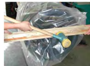
Figure X-g – Avoid Contamination During Installation
