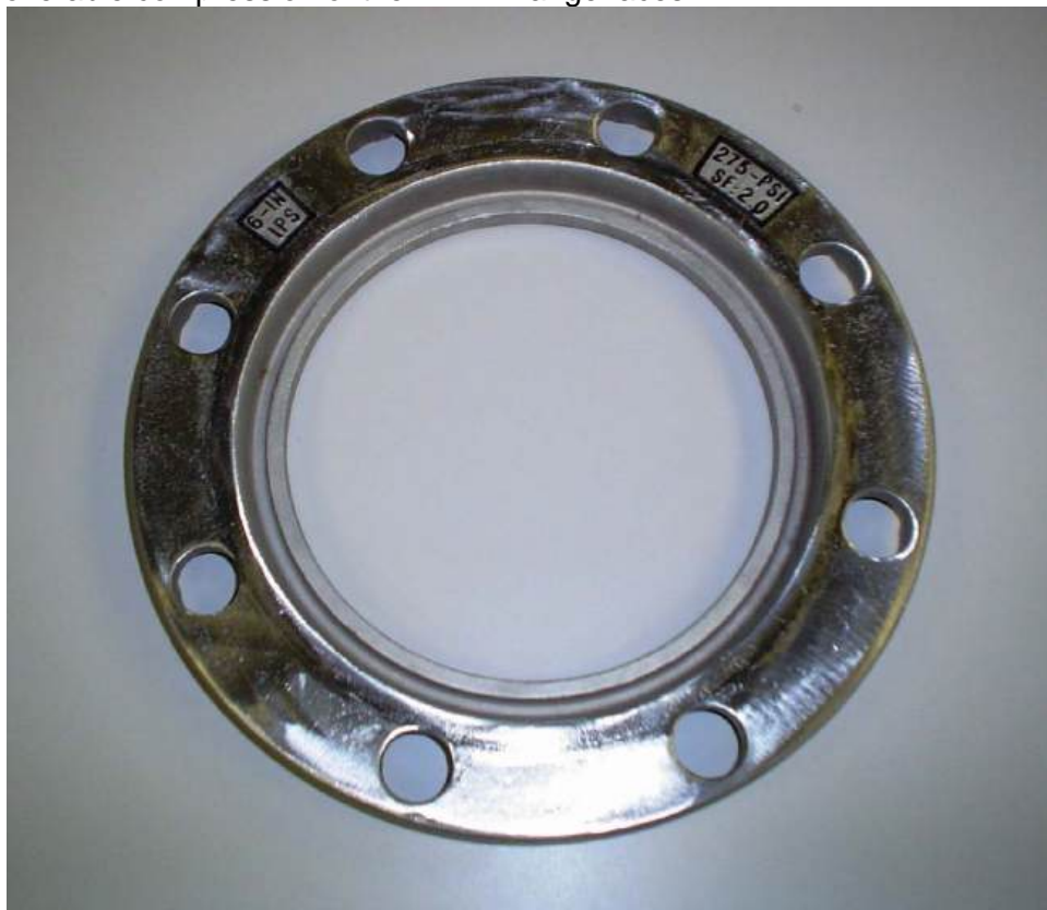
Figure 4 Cast Stainless Steel, Lap-Joint Flange, 6-inch IPS
