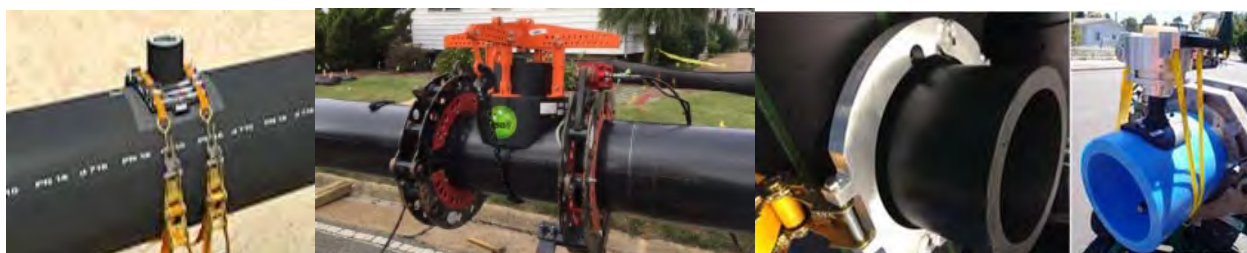
Figure VI-c - Reusable saddle clamps
