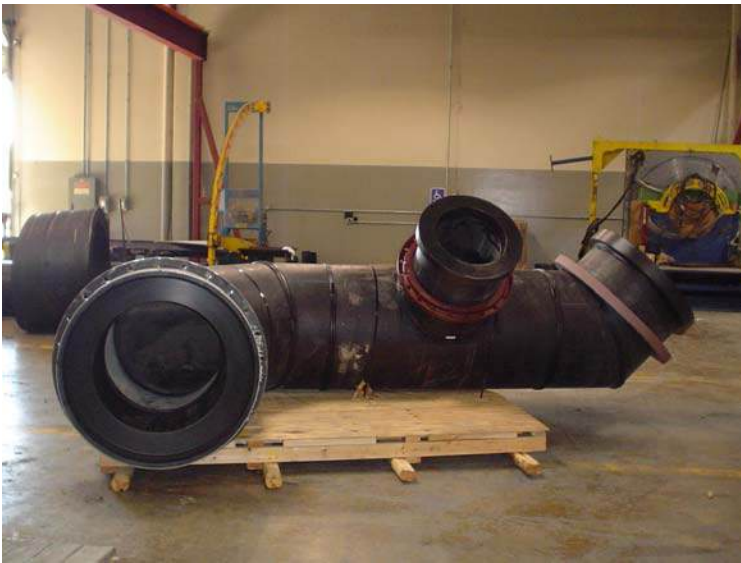
Figure 7 Fused Manifold Assembly with Flange Adapters And Back Up Rings
