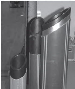
Figure 22 Protecting the PE Pipe from Shards
