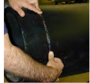
Figure IV-a - Measuring pipe diameter with Pi tape
