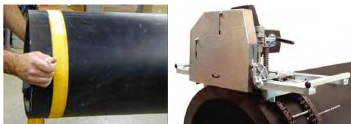
Figure III-c – Marking and cutting larger diameter pipes
