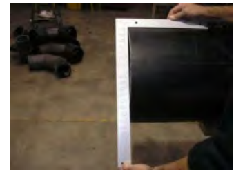
Figure IV-b - Measuring allowable gap with Carpenter's Square
