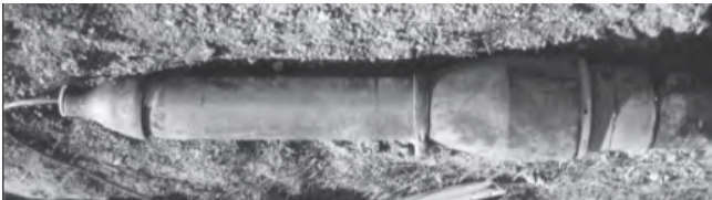
Figure 2 The Bursting Head of the Pneumatic System
