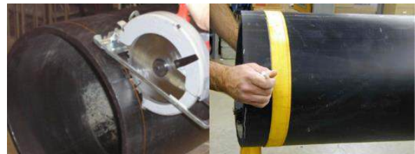
Figure IV-d – Marking and cutting larger diameter pipes
