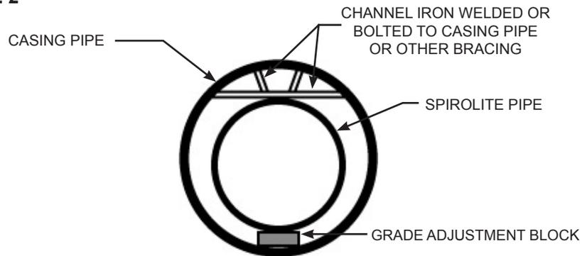
TYPICAL FIXED RESTRAINING SYSTEM ATTACHED TO CASING
